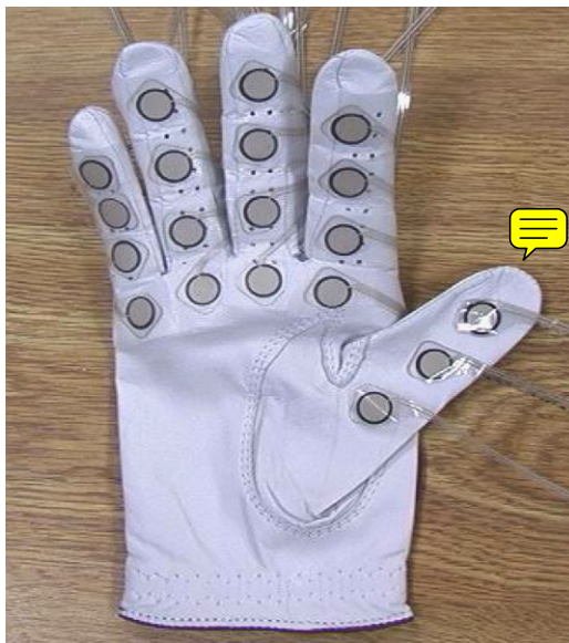
Fig. 2. FlexiForce TM sensors outfitted on a glove used for measuring hand force.
